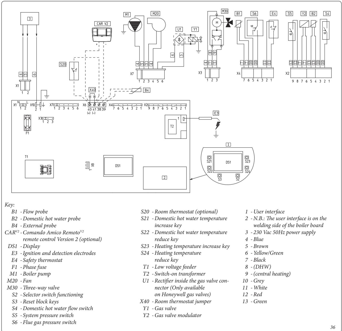
The boiler is designed for application of a room thermostat (S20), an On/Off room chronothermostat, a program timer or a Comando Amico Remoto<sup>V2</sup> remote control (CAR<sup>V2</sup>). Connect to clamps 40 - 41 eliminating the jumper X40, paying attention not to invert the polarity if the CAR<sup>V2</sup> is installed.
